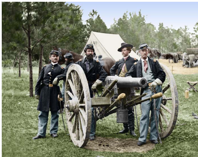
Mosby used a 3-inch ordinance rifle like this one on August 24, 1864. It was very accurate within a range of 2,000 yards and fired an elongated solid shell.
