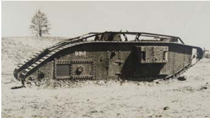
The 301st Battalion, Tank Corps were supplied with British Mark V tanks with "unditching beams" similar to the one above.
