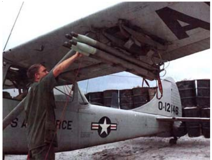
USAF Airman inspecting 2.75 inch white phosphorus smoke marking rockets on an O1 Bird Dog, Vietnam c. 1967.
